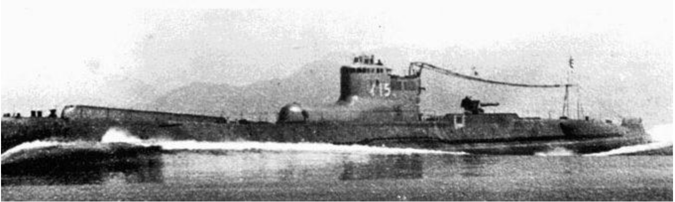
Imperial Japanese Navy Submarine I-15. Note bulge in front of conning tower for aircraft stowage
